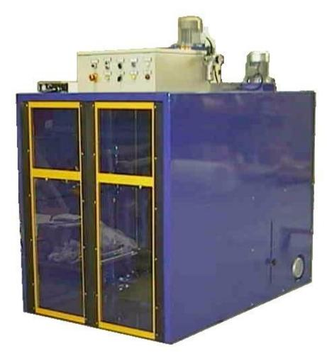
Automatic painting machine with tyre loading and unloading from the same door. The system uses conical rollers for centering the tyre and is equipped with an electric fan. The machine is ATEX certified zone 2 and 21, suitable for painting tyres from 16" to 24".
