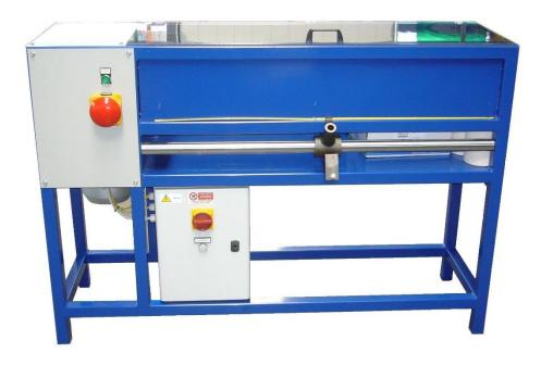
Equipment for manual cutting of rolls of substrate, calendered or side leaf. Positioning takes place by means of a manual knife following a position indicator (meter). The rotation is done by means of a gearmotor controlled by a pedal and locking by a manually expandable shaft.
