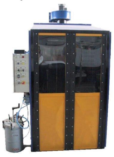
Automatic painting machine with tyre loading and unloading from the same door. The system uses conical rollers for centering the tyre and is equipped with an electric fan. The machine is ATEX certified zone 2 and 21, it has the possibility to paint the sides of a small earth-moving machine up to a maximum of Ø1700 and width 700.
