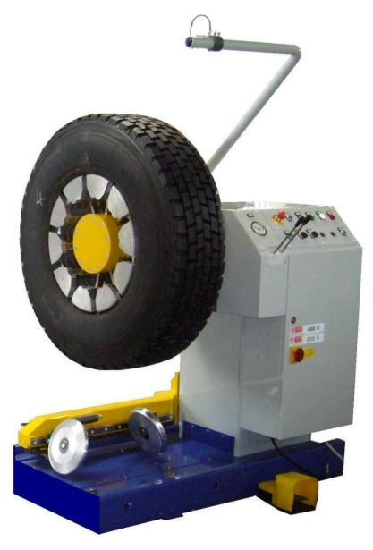
Manual packaging and rolling machine with interchangeable mandrel. The machine is equipped with a hydraulic unit for opening the spindle and rolling, the packaging in this case is done by hand by rotating the tyre with the pedal and centering the tread with the reference laser pointer. The rolling cycle is automatic.
