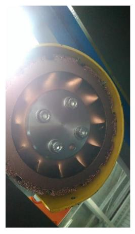
Machine for grinding the PCT pre-molded tread head with a locking system and a pneumatic cylinder. The starting of the grinding wheel takes place by means of a two-hand control with the possibility of adjusting the depth of cut with a handwheel.
