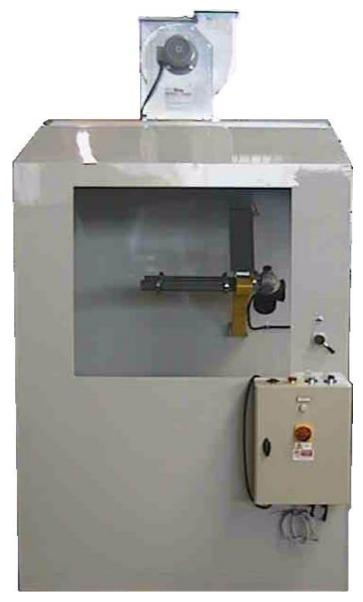
ATEX certified cementation cabin to be inserted in the monorail with pneumatic lifting system for the extraction of the hook, compressed air frame system around the window to prevent the escape of gases generated by the spray of the gun. Pneumatic control for lifting the arm and pedal for rotating the tyre.
