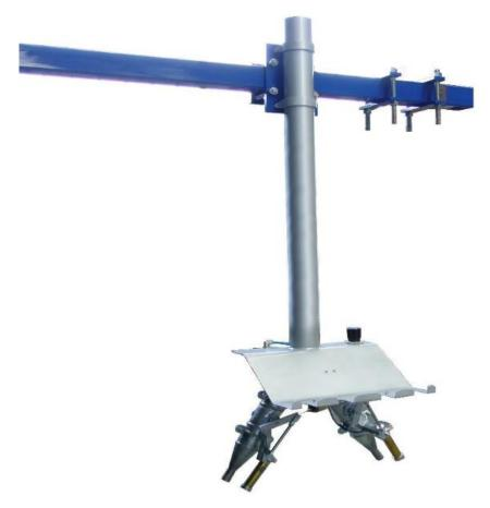
Support to be applied to any monorail to deposit all the tools for the operators of the crater stations, connectable to the suction system. The opening of the suction ducts is activated only when the operator removes the tool to be used from its housing. There is also a pressure regulator for the correct pressure for the tools.
