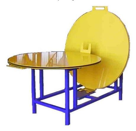
Tilting table on both sides and rotating discs for the assembly of envelopes.
