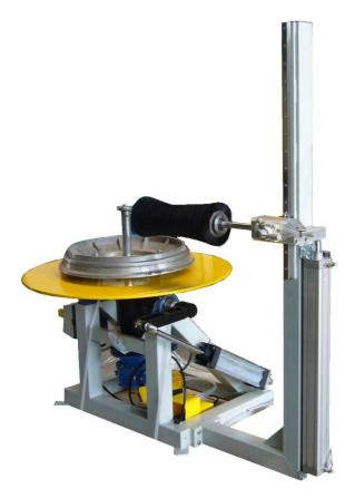
System with tilting table controlled by a pneumatic cylinder and central bead for centering the tyre. The rotation takes place by means of a pedal control. There is also a pneumatic cylinder with a rigid bristle brush to help roll the side leaf.
