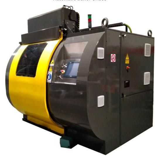
Automatic buffing machine for truck tyres from 16" to 24", with automatic tyre loading, interchangeable beads, laser circumference measurement system, double motor brush group, material evacuation system by means of a screw, removal of the tread by means of a cutter and basket to perform the necessary roughness (RMA) with minimal removal.
