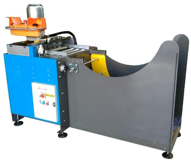
Machine for grinding the PCT pre-molded head with a pneumatic cylinder locking system and the starting of the grinding wheel by means of a two-hand control. The depth of cut is adjustable by means of a handwheel. The machine has a roller conveyor for loading the roll of pre-molded tread that can be moved to a convenient position for use by means of a pneumatic cylinder system.
