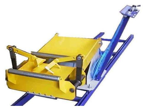
Manual inspection system for checking and repairing tyres on monorail with controls and movements through pneumatic cylinders.
