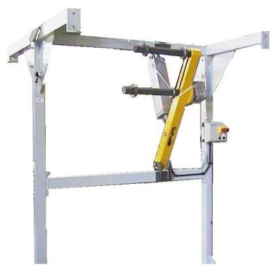
Crater station to be coupled to a monorail or can be used individually with mobile arm operated by a pneumatic cylinder. The rotation control of the pneumatic traction pedal takes place via a gearmotor for each roller.
