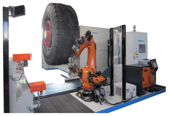
Robot system for processing craters and repairing OTR tyres from 24" to 63" with expandable spindle locking system, KUKA anthropomorphic robot, liquid-cooled electro-spindle including chiller, 9-position tool rack with automatic guards, nets and gates protection, joystick system for identifying defects to be machined and the possibility of repeating a machining program with a programmable step.
