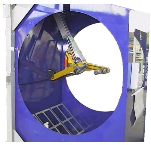
Cementation cabin to be inserted in the monorail with pneumatic lifting system for the extraction of the hook, compressed air frame system around the window to prevent the escape of gases generated by the spray of the gun. Pneumatic control for lifting the arm and pedal for rotating the tyre.
