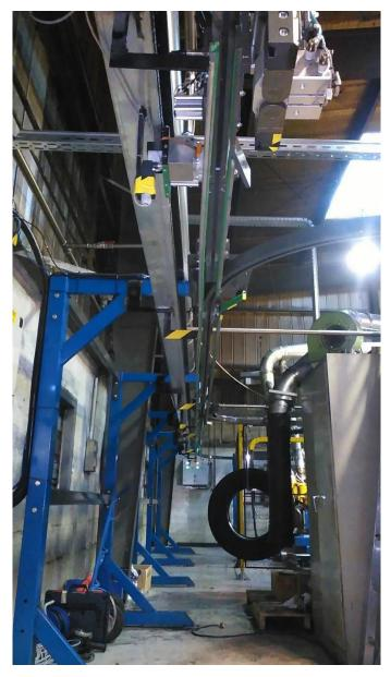
Automatic system for the enslavement of the CT4.0 crater robot. The operator accumulates the freshly buffed tyres on a straight monorail, the shuttle automatically searches for the first hook and with a chain system delivers it to the CT4.0 crater robot (in the photo there is a 10m straight version but curves or rings are also available).
